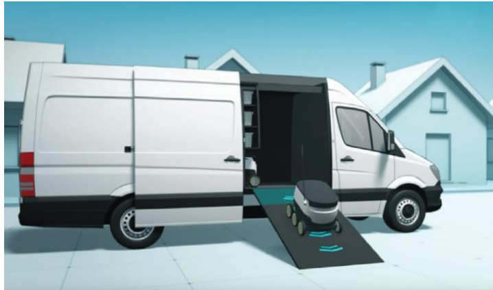
FIGURE 36 - SPECIALIZED TRUCK LAUNCHING ROBOTS AT THE CURBSIDE.
